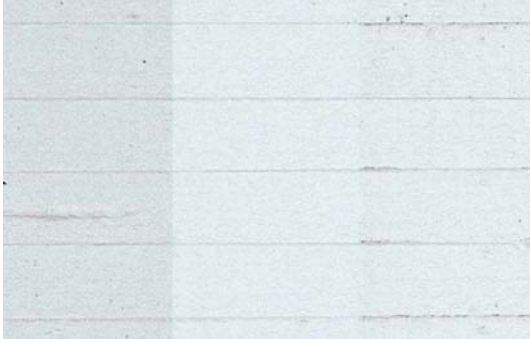
The StoLotusan test surface (middle) remains discernably cleaner than the two facade paints on the left and right.
