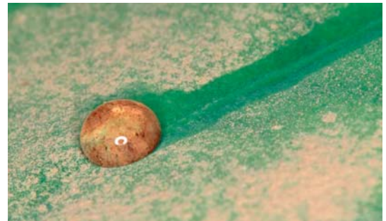
On the microstructured, super-hydrophobic StoLotusan surface water droplets take on a spherical form, pick up the dirt particles which are only loosely deposited on the surface and leave a clean trace in their wake.
